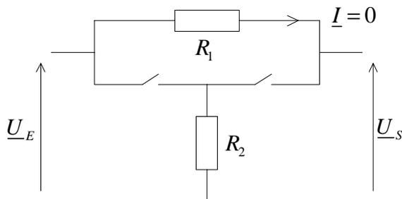
$$\underline{U}_S = \underline{U}_E \Rightarrow \underline{H} = 1 \text{ ou } H_{dB} = 0$$
